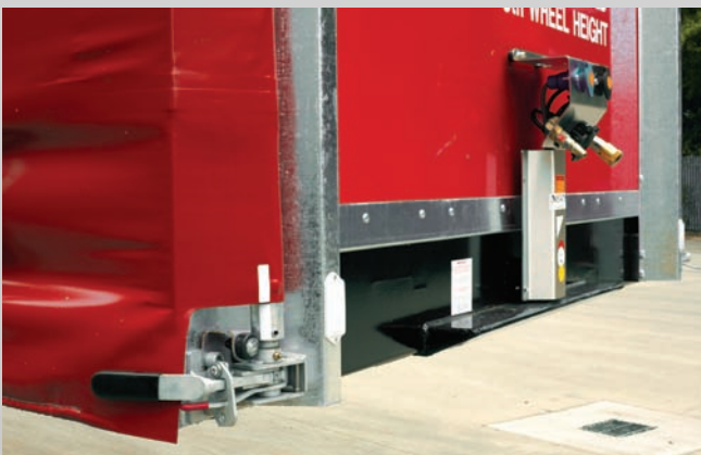
Galvanized front pillars, ratchet tensioners, raised coupling box.
