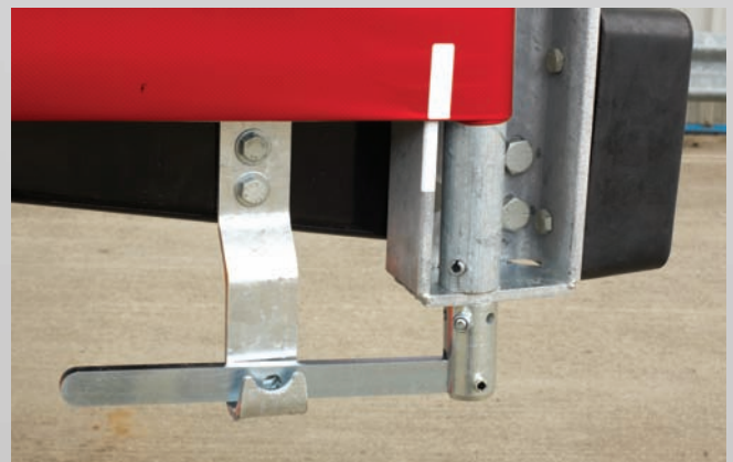
Rear tensioners, galvanized posts, heavy duty block buffers.
